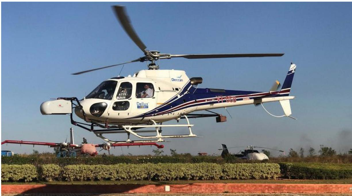
Figure 1: A helicopter equipped with Light Detection and Ranging system.
